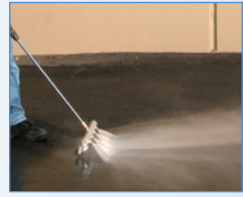
Spray action of the Water Broom
