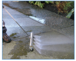
Spray action of the Water Broom
